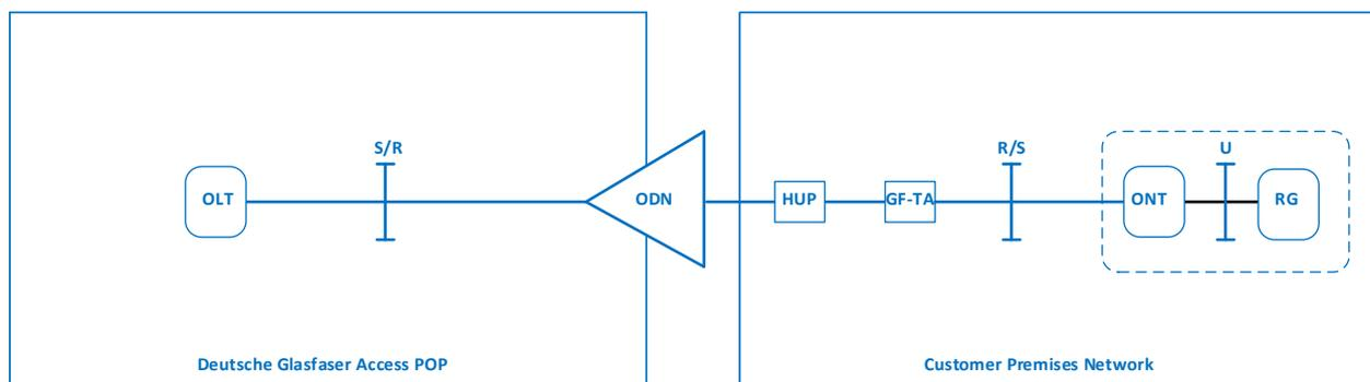
$IF_{PON}$  denotes the interface at reference points S/R and R/S. This interface must support all protocols that are necessary for transmission between OLT and GPON and XGS-PON ONT's/ONU's.
